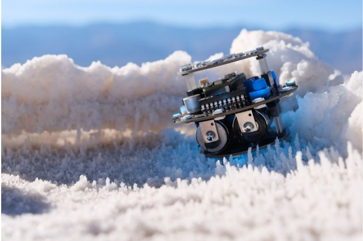
Speculātor unit without enclosure installed at Badwater Basin, Death Valley, California.
