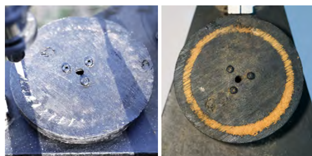
Figure 8: Explorator chipper ’s wooden turntable showing minor(left) and major (right) damage.
